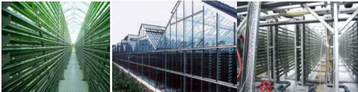
Figure 3. IVG Photobioreactors in Kloetze, Germany (appx. 1 ha of greenhouses)
